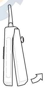
1a. If you are going to use alkaline batteries, remove the alkaline battery compartment cover and install 6 AA alkaline batteries. Re-install the cover to the battery compartment, then secure in place.
